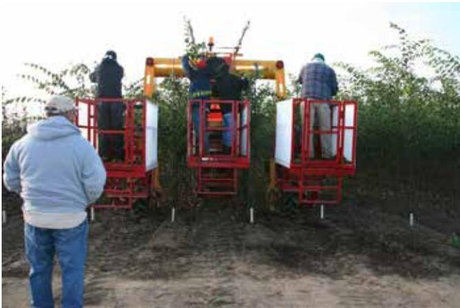
Featured in the PlantLine previously, the Damcon Multi-trike has been a centerpiece in multiple focus groups. Recently, fall topping (i.e. pruning), a skilled, labor driven task, was challenged in a focus group to improve efficiencies and immediately ideas swarmed around the Damcon due to its ability to tackle multiple rows with a single pass.
