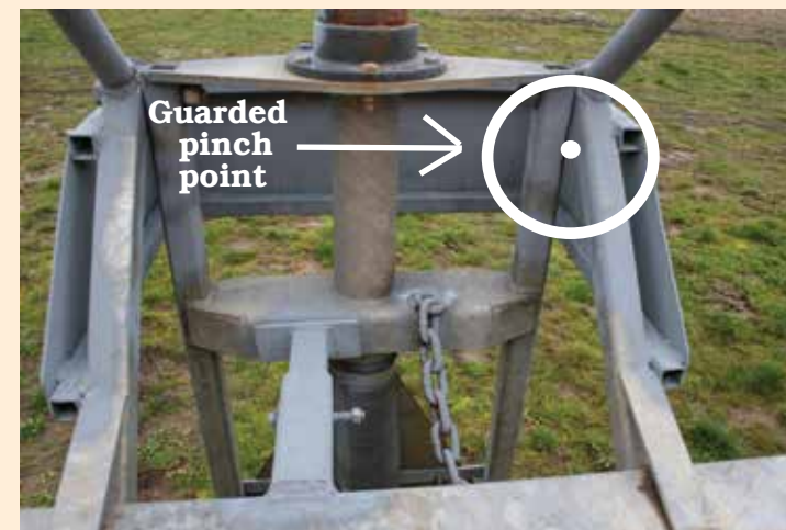
Close up of guard, block and chain
